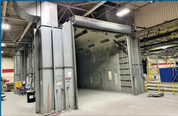
28' W x 45' L x 16' H Pass Thru Paint & Cure Booth
