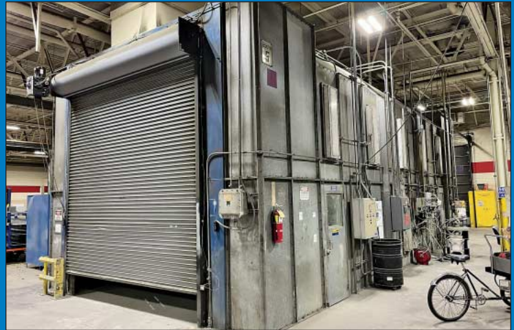
20.5' W x 43' L x 16' H Pass Thru Paint & Cure Booth
